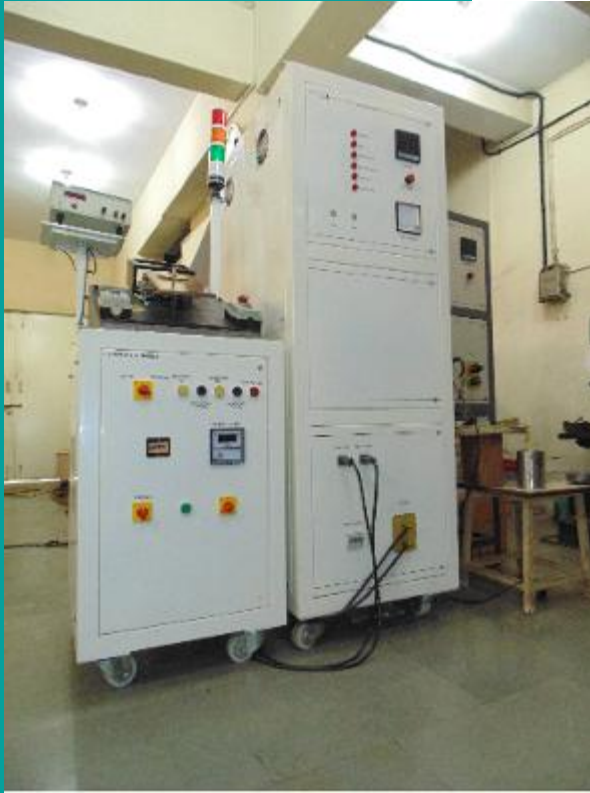
Magnetizer with Peak Current measurements and Pneumatic system with automatic operation and Magnet strength checking with each operation
